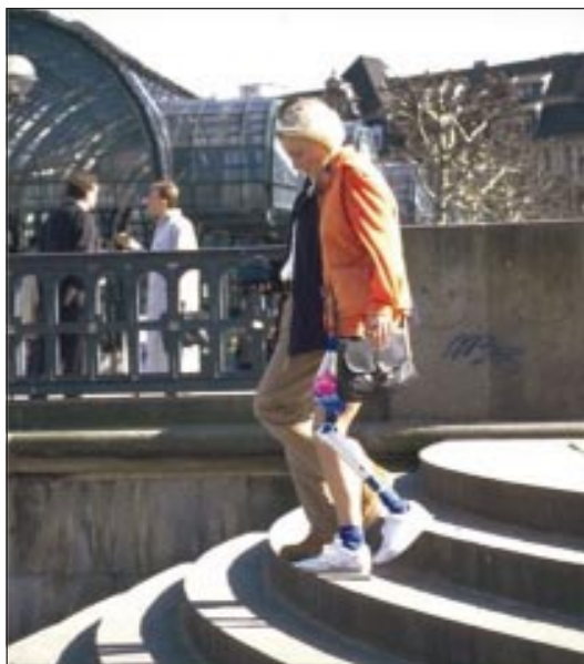
Fig 4 The Otto Bock C-Leg with computer controlled knee and integrated motion and force sensors to optimise hydraulic damping, making both walking and stair descent easier. (Picture courtesy of Otto Bock)
